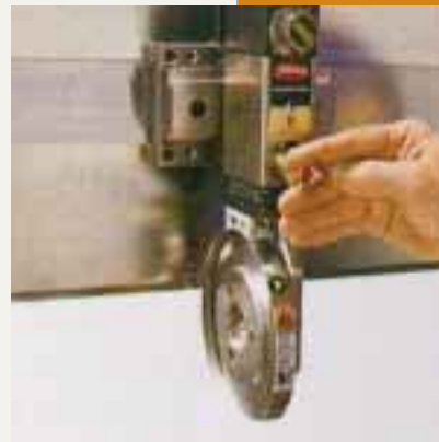
Photo 1: The ability to reverse the cant angle is easily accomplished by rotating the cant-control key in this unit. This allows slitting on the opposite edge of the lower slitter ring. No tools are required.
